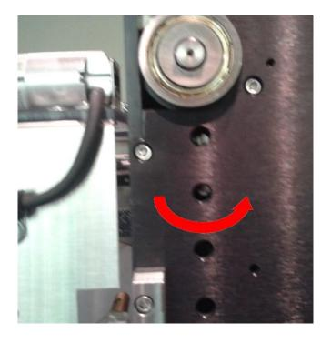
Turn the Bottom Shaft Counter-Clockwise a 1/2-turn.
